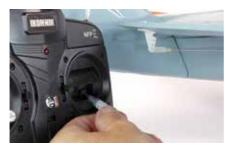
12. With motors still in the forward flying position move the aileron stick to the right and check that the right-hand elevon moves in an upward direction whilst the left-hand elevon moves downward. Moving the aileron stick to the left will have the opposite effect.
